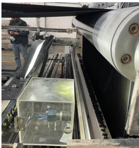
Figure 4 - Placement of the camera in housing prototype-4
