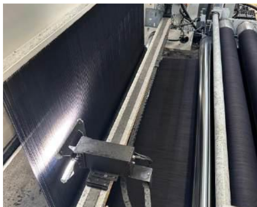
Figure 9 - Placement of the colour detection system
