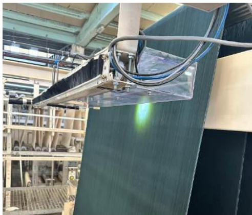
Figure 3 - Placement of the camera in housing prototype-3
