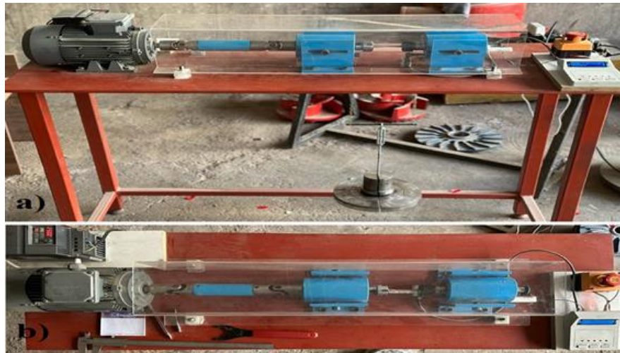
Figure 8. Rotational bending fatigue test device manufacturing drawing a. front view b. top view
