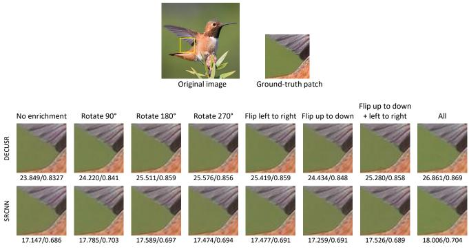
Figure 5. The performances of models in PSNR and SSIM measures. Subfigure on left is for DECUSR (a) whereas subfigure on right is for SRCNN (b). The numeric values shown below the images show the PSNR and SSIM scores.
