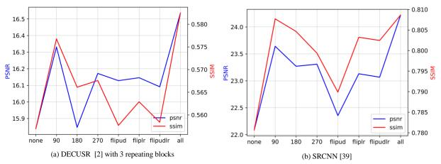
Figure 4. The performances of models in PSNR and SSIM measures. Subfigure on left is for DECUSR (a) whereas subfigure on right is for SRCNN (b). The abbreviations for flip operations as follows; lr: left to right, ud: up to down, udlr: up to down plus left to right. None indicates training with original dataset wihout any enrichment.
