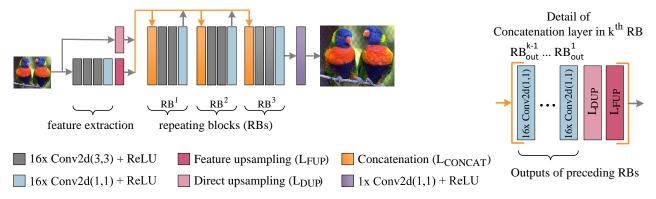
Figure 3. Architecture of DECUSR [2] model with three repeating blocks.
