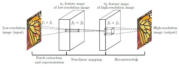
Figure 2. Architecture of SRCNN [39] model.
