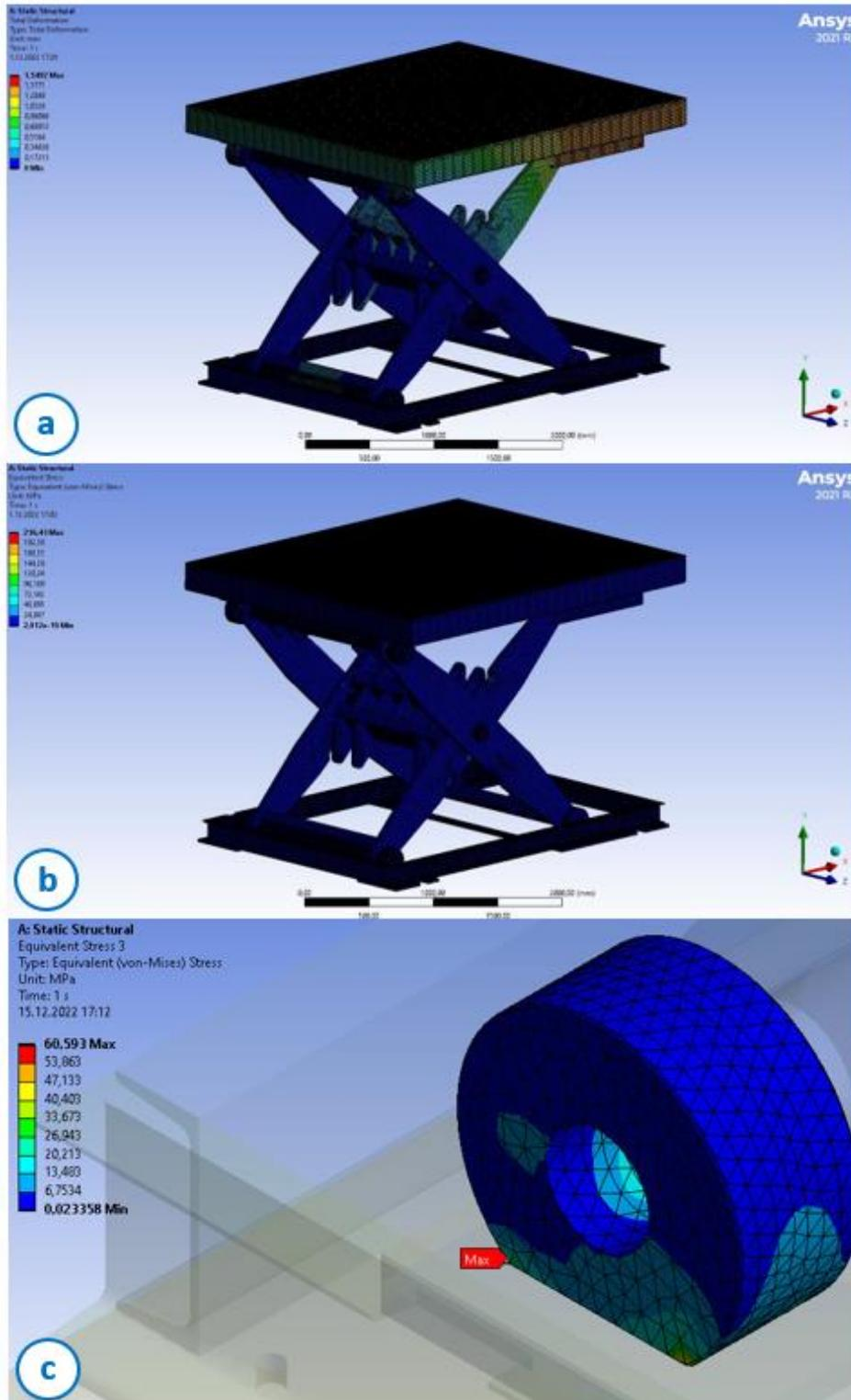
Figure 3: a) Total Deformation Analysis of Scissor Lift Platform, b) Von-Mises Stress Analysis of Scissor Lift Platform, c) Von-Mises Stress Analysis of Bearing Hinge System
