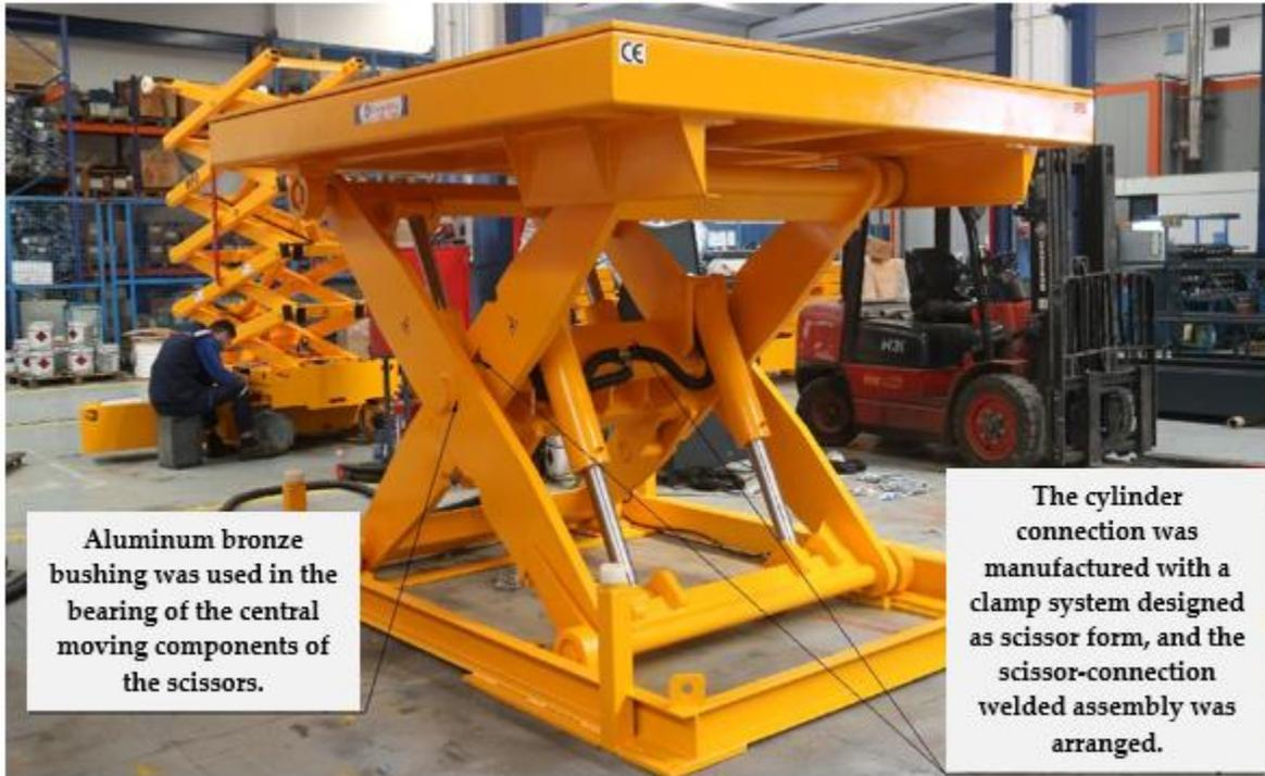
Figure 5: Prototype with Innovative Clamp, Bushing Bearing and Guiding System
