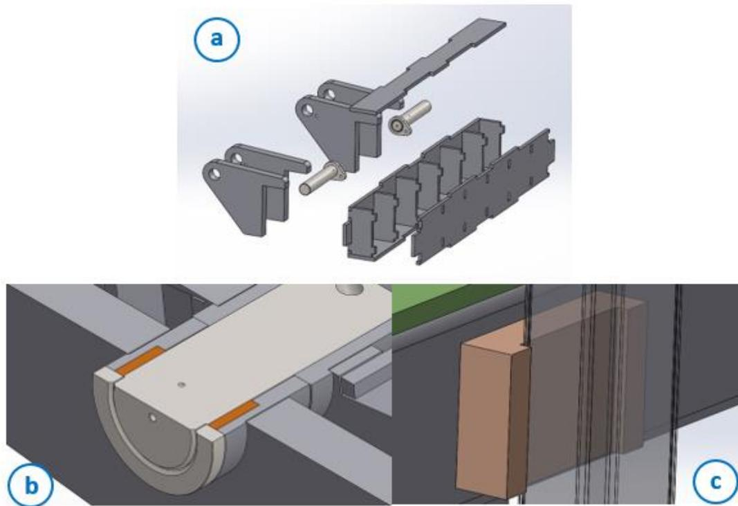
Figure 4: Solid Models of a) Innovative Connection Assembly Clamp System b) Aluminum Bronze Bushing Bearing Assembly c) Aluminum Bronze Guiding System
