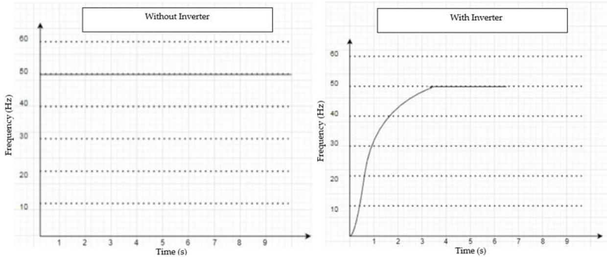
Figure 8: Frequency-Time Graph of Electric Motor a) Without Inverter, b) With Inverter
