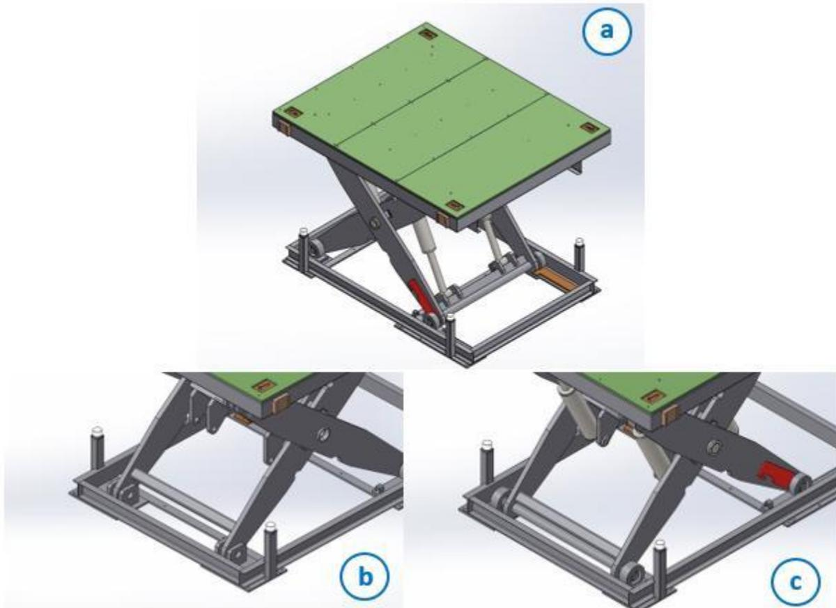
Figure 1: a) Innovative Scissor Lift Platform 3D Solid Model, b) Conventional Welded Hinge-Scissor Model, c) Innovative Bearing Hinge-Scissor Model
