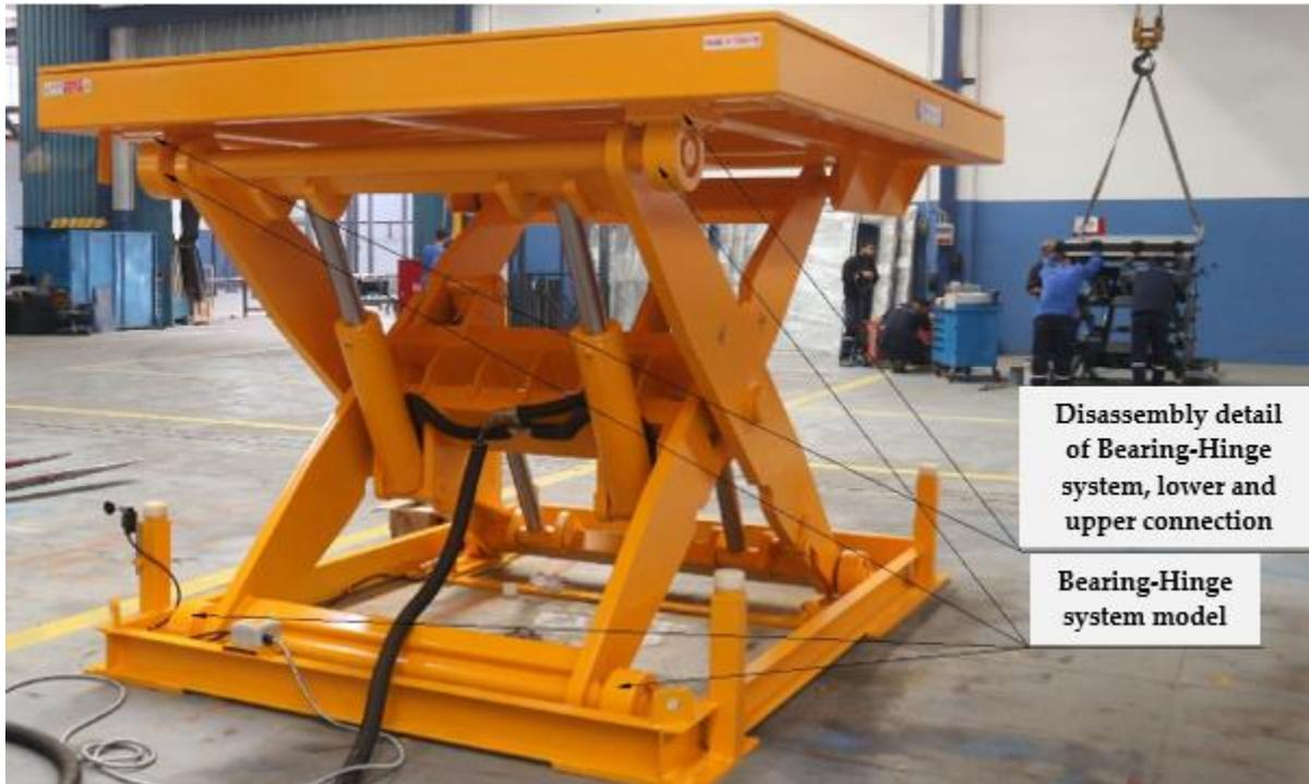
*Figure 2: Prototype with Innovative Bearing Hinge-Scissor System*
