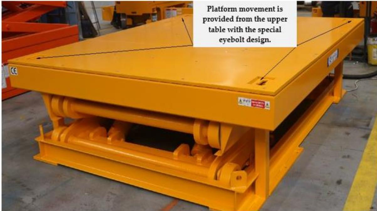
*Figure 7: Appearance of Eyebolts Design on Prototype*
